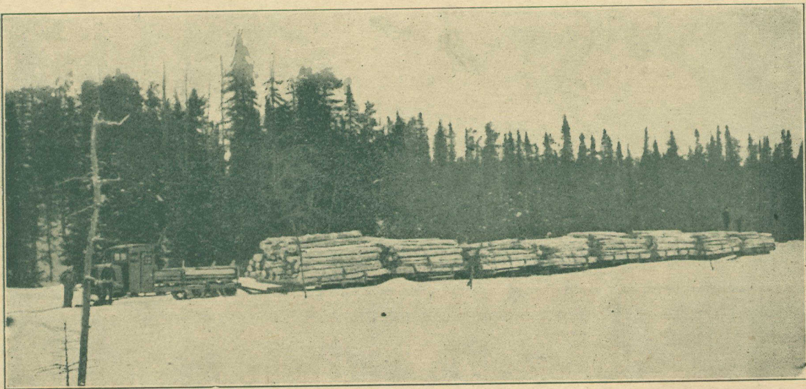
Linn Logging Tractor on Operation of Austin and Nicholson Ltd., Esher, Ont. Hauling distance 7 miles—maximum days hauling—2885 logs equivalent to 225 cords.
