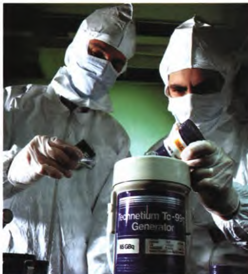
Nordion's Technetium-99 generators for drawing off sterile radiopharmaceuticals used in diagnostic tests.
