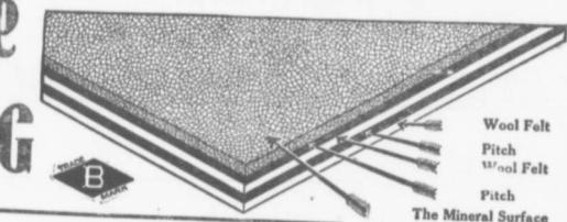
Most roofings are made of only one layer but Amatite is made in Five Layers. The bottom layer is wool felt, the next is real Coal Tar Pitch, the third is wool felt, the fourth is pitch again, into which is embedded the fifth layer, namely, the Mineral Surface.
