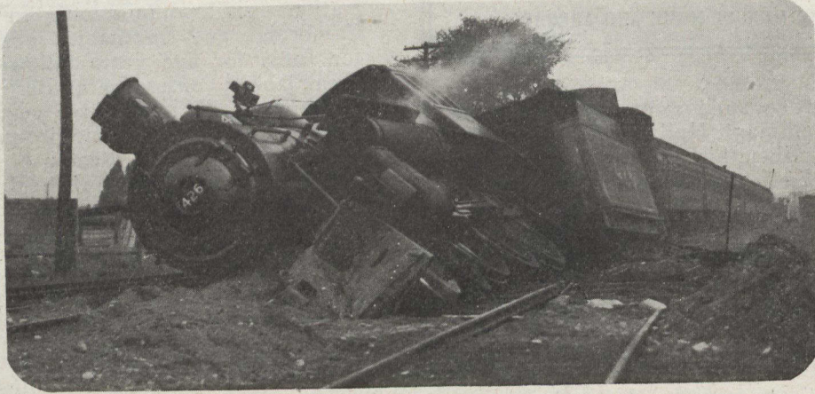
What happens when some hoodlums interfere with a switch "point." This particular accident happened to the North Bay train while entering Toronto.
