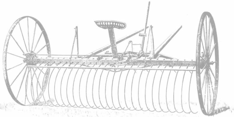
The Frame may be at an angle of 40 degrees, but the Bar still adapts itself to the necessity. : : :
