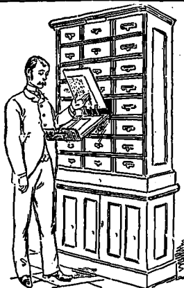
Shannon Filing Cabinet on base, showing how papers may be examined without removing drawer.
