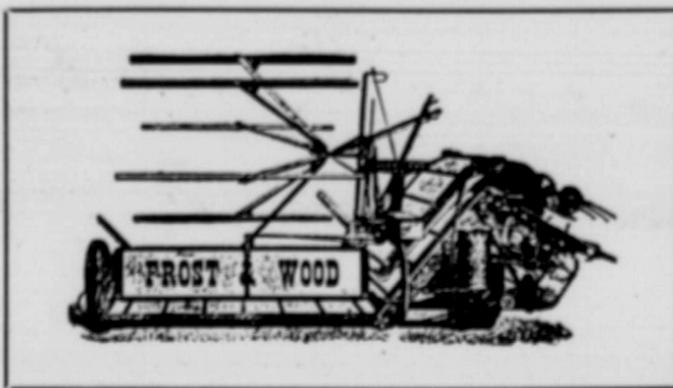
The top elevator roller is set so far forward the grain is carried till it is on the downward drop.
