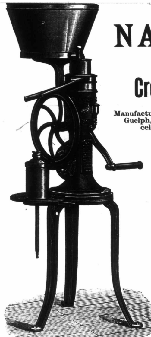
"NATIONAL" NO. 1 HAND POWER. Capacity, 330 to 350 lbs. per hour.
