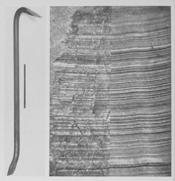
Left: The incriminating crow-bar found on the Frank farm. Right: Photomicrograph comparing (left) part of tool markings on metal lining of safe door with (right) crow-bar markings on test metal; note how striae on both plates conform.
