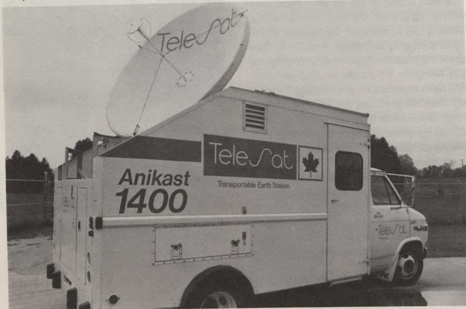
The van-mounted transmitting service can put a broadcast crew on the air within 20 minutes.
