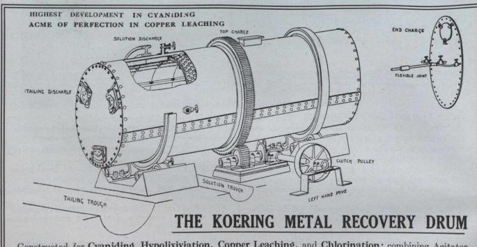
Constructed for Cyaniding, Hypolixiviation, Copper Leaching, and Chlorination; combining Agitator Filter, and Washer. Highest extraction in shortest period of time: saving labor. power, and chemicals.
