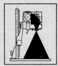
does not go straight from lamp to negative, but is deflected downwards by a mirror. Heat escapes not only through lamphouse vents but also from back of mirror. Lamp may be raised and lowered, as well as rotated to ensure precise centering with mirror. Illumination is totally even, yet retains the crispness of a condensor enlarger.
