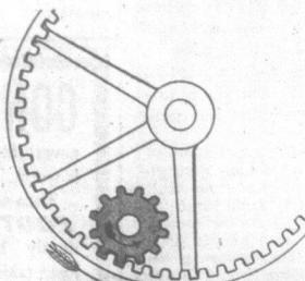
This is an external gear used on other mowers. Do you see the difference? These two wheels don't agree together so well. They have opposite tendencies. The big wheel scratches and scrapes at the little one and the little one tries hard to get away from the big one.
