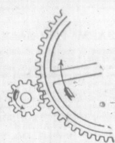
The Internal gear is better, too, because there are more teeth in contact at the same time and the teeth are more fully meshed, hence more even wear and less wear—greater durability.
