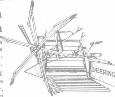
The third discharge arm on Deering Binders is very effective in throwing out the bound sheaves, and in addition to this it assists in separating the tangled grain of the bound sheaves from the unbound grain on the binder deck. The binder shifter lever, directly in front of the driver, is convenient to operate.
