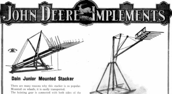
The hoisting gear is connected with both sides of the stacker head. The head does not sag or tilt while being elevated, letting the hay slip off.
