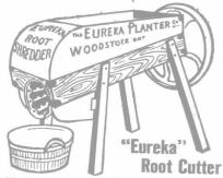
will slice or shred from 1 to 2 bushels per minute. Fastest machine made—easiest running. Tapering cylinder—10 best steel knives.
