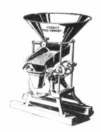
THE Vessot "Champion" cleans grain as well as grinds it. The spout that carries the grain to the grinder is made with two sieves, a coarse one above and a fine one below. The coarse sieve catches nails, sticks, and stones, but lets the grain fall through. The fine sieve holds the grain, but takes out all sand and dirt. The grain passes to the grinding plates as clean as grain can be.
