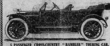
5 PASSENGER CROSS-COUNTRY "RAMBLER" TOURING CAR. This smooth running car is electrically started and lighted; has 120 in. wheel base; long stroke 38 h. p.
