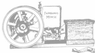
This cut shows our One-H.P. Jack Junior Engine. Not an air-cooled toy, which is forever giving trouble, but a simple, practical, durable, water-cooled engine, that can be relied upon at all times. Just the thing for pumping water, running separators, churning, washing machine, ice-cream freezer, or any other such purposes.
