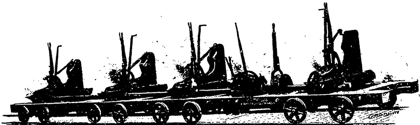
FOUR BLOCK CAST STEEL CARRIAGE WITHOUT AUTOMATIC COUPLER.
