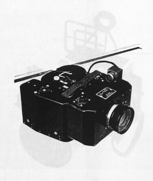
Figure 8. The Vinten Type 1360 reconnaissance camera complete with automatic exposure control and 6 inch lens. The film magazine holds 500 exposures on 70 mm film. (Source: Graham, Ron and Roger E. Read. 1986. Manual of Aerial Photography. Focal Press. London. p. 44.)
