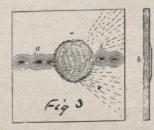
About the only perfect tooth appears to be at a and b, but it is comparatively easy to make new teeth for this saw. A case of severe jointing and the saw will be made round. Then the teeth may be spaced better and the spacing gradually improved by each and every filing or grinding. It does not pay to file saws, nowadays; files cost much more than emery wheels, and the use of a good emery grinder would
