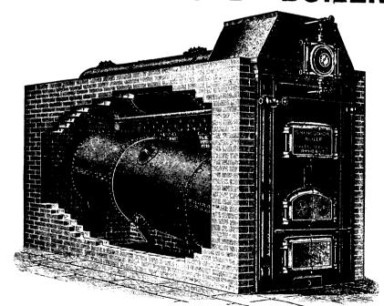
Is built for brick casing, or with sheet steel case, as desire by purchaser. Uses 10 to 25 per cent. less coal than a return tubular boiler.
