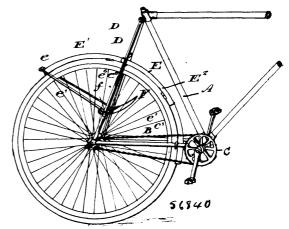
the lugs  $e^{a}$  and  $e^{7}$  when the sections are extended, and means for holding the extended sections in position upon the frame, as and for the purpose specified.
