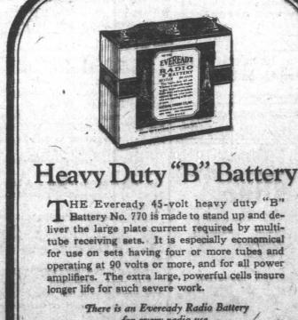
Battery No. 770 is made to stand up and deliver the large plate current required by multitube receiving sets. It is especially economical for use on sets having four or more tubes and operating at 90 volts or more, and for all power amplifiers. The extra large, powerful cells insure
