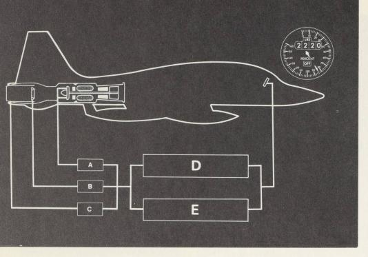
The system, which will be flight tested in the near future, will consist of gasflow sensors mounted on the aircraft engine and an airborne special purpose computer for calculating actual thrust of an engine. The calculation will appear on a cockpit indicator in front of the pilot. The computer also has to calculate the thrust which the engine should be capable of developing if properly operating.
