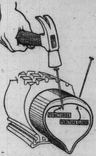
Here, at last, is an air tube that you can puncture, remove the cause of the puncture, and no complete hole remains to allow the air to leak out. Simplex Puncture-proof Tubes are pneumatic tubes that will positively not leak, thus preventing your tires from sagging and consequent rim-cuts, stone bruises and blow-outs-in short, a perfect inner tube that will do more than the ordinary tubes, without being subject to their worrisome defects.
