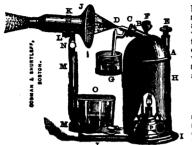
Fig. 15. The complete Steam Atomizer.
