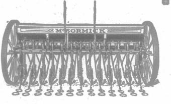
The angle steel main frame, removable scrapers, and folding levers all add to the durability and satisfactory service of McCormick drills.
