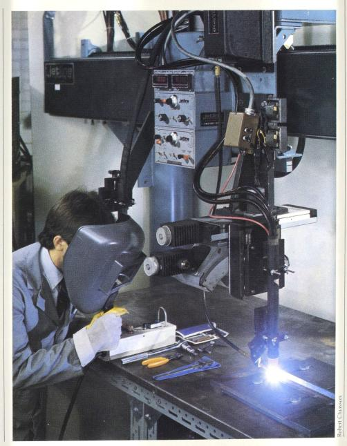
Not a robot, but close: this commercial welder needs no human intervention during actual welds, provided its operator sets necessary parameters before welding begins. Capable of performing both gas-tungsten and plasma-arc welding, the system is like those used to weld aluminum plates for the U.S. Space Shuttle.
