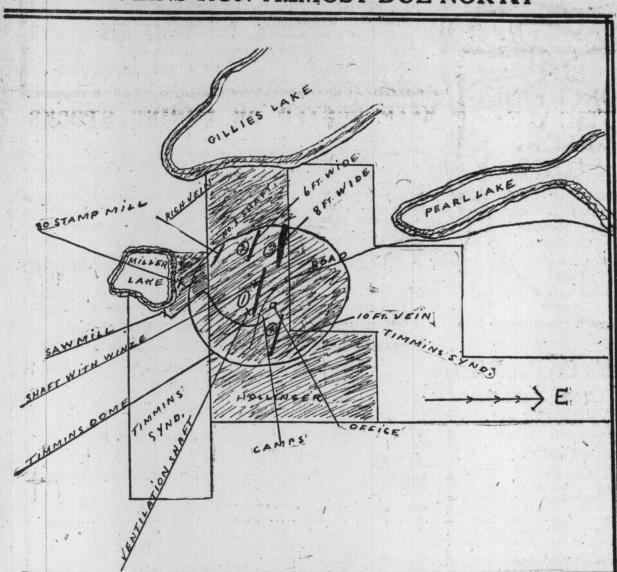
The above plan shows the workings and veins on the Hollinger property. The veins are indicated as follows: (1) Original Timmins' vein, known as No. 1. The vein is 700 feet in length between the portions marked X. (2) Quartz outcroppings, which indicate they belong to the No. 1 vein, which butts into the schist 26 feet west of the No. 1 shaft. Showings here as rich as in No. 1 vein, have been made. (4) Quartz outcropping to be developed this season.
