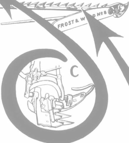
Illustration C shows you the Large Bearings used in our "stay-tight" connection between Cutter Bar and Main Frame of Mower. Unlike Small Pins used on other mowers, they do not wear down hurriedly and permit connection to work loose. Instead, they fit precisely together and have no chance to wear. That's why it is called the "stay-tight" connection. That's why there is no time lost on the field—no blacksmiths' bills to pay.
