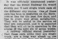
truck, are a long way ahead on the single truck cars that are in operation at the present time. A steel under-frame is used through, which gives the car greater strength, while the adation of a longer rear platform, elec-tric bell service, and a wider front dour entrance, makes the new car a distinct innovation. The cars are equipped with the Teacock brake, which is considered to be the best for this class of car. The air brake has never given entire satis-
