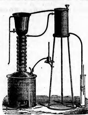
Apparatus "de Precision" to determine the Alcoholic richness of Wines.
