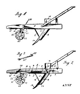
depending lever 19, formed with the eye 18, and toe 21, the co-acting ground wheel having pins and the pivoted latch adapted to engage said lever, substantially as and for the purpose set forth.
