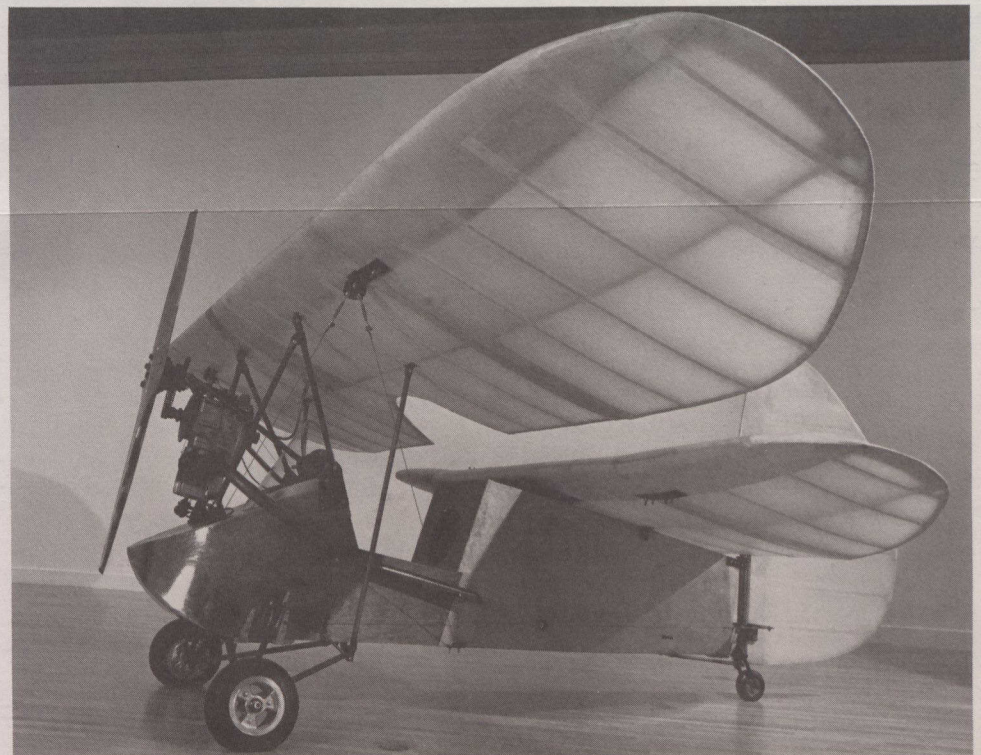
The Flying Flea (1976-77) made of plywood, wood, steel, cloth, glue, aircraft dope, varnish, paint, engine and wheels. (216x545x399 centimetres).
