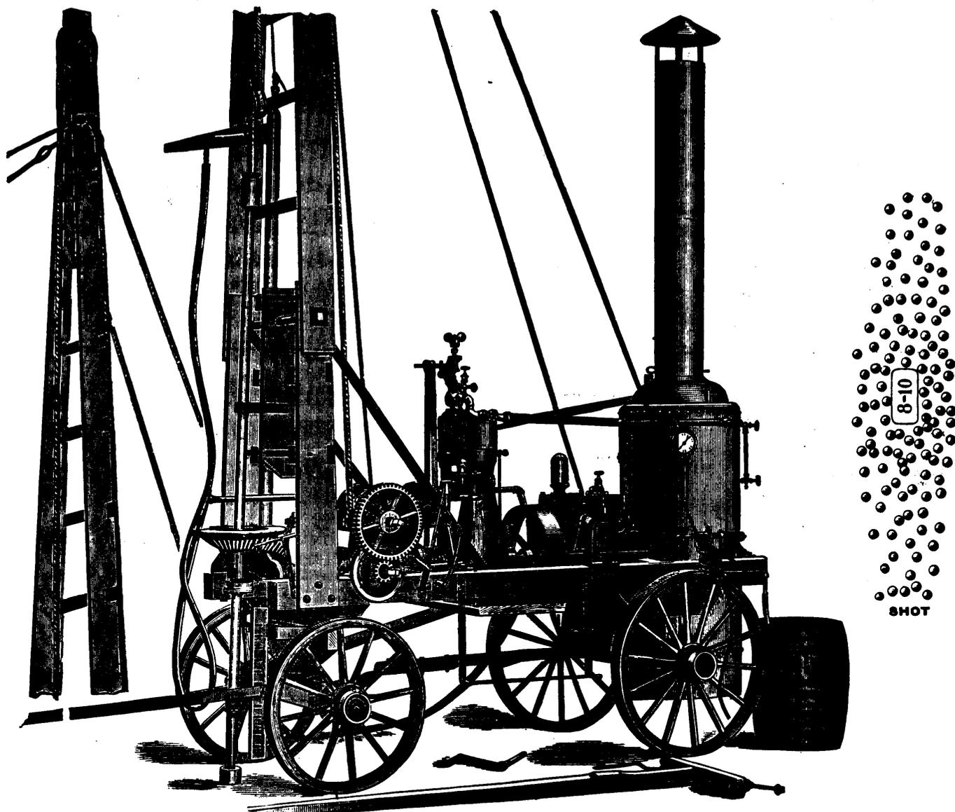
**T**HIS DRILL does the work without the use of Diamonds, using as a substitute Chilled Steel Globules, or as they are commonly called, shot. These are inexpensive, costing in actual work about ten cents per day; whereas, diamonds are very expensive, a single one often costing from \$30 to \$100, thus showing the difference in cost in case of loss of tools. It is THE BEST, CHEAPEST, and MOST EFFECTIVE CORE DRILL made for Prospecting Quarries, Coal Lands, Sinking Wells and the like.
