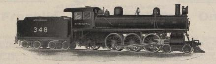
Pacific Type Passenger Locomotive built for the Intercolonial Railway. Total weight of engine, 194,500 pounds. Weight on driving wheels, 132,000 pounds; diameter of driving wheels, 72 inches. Boiler pressure, 200 pounds. Maximum tractive power, 29,200 pounds.
