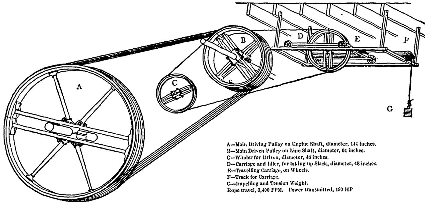
A—Main Driving Pulley on Engine Shaft, diameter, 144 inches.
