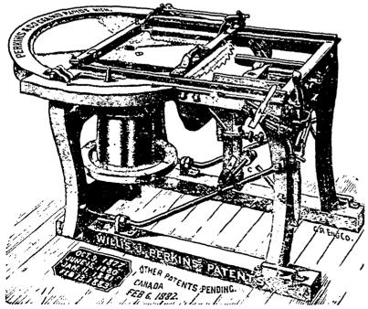
The only Herizontal Saw Machine on which a thick slab can be cut from the bolt. SECOND CUT ALWAYS A SHINGLE. Knots, total hearts, but squared rift ways, and all irregularities cut off at one clip. This improvement will pay price of the whole machineevery season by increase of quality and quantity cut.
