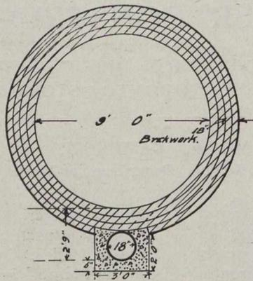
Fig. 3.—Brick Section in Tunnel.
