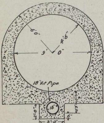
Fig. 2.—Concrete Section in Open Cut.
