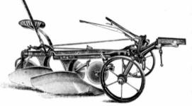
This is a Double Plow, used for general purposes and cutting two furrows from 9 to 12 inches as desired and can easily be regulated for sod or stubble.
