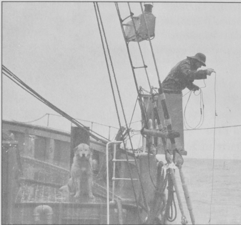
Sounding with the lead line from St. Roch.
