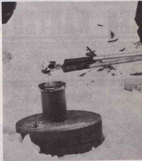
(Left) the pieces of the puzzle start to come together. (Right) using long tongs, a scientist places bits of radioactive debris in a lead container.
