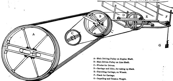
The illustration, as shown above, is one of peculiar construction, and represents an engine transmitting its power to the line shafting by the Potent System of manilla ropes and grooved hardwood pulleys. Transmissions similar to the above are now in use at the works of the following well-known manufacturers in Toronto: manufacturers in Toronto
