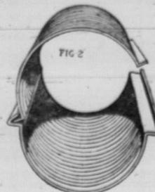
Note that the ribs are flat, and the curved part of the cylinder deeply corrugated. These ribs add vastly to the culverts' strength. Unskilled labor, with a simple
