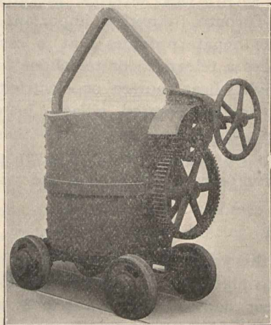
New Works of Sturtevant Co.—Two-ton Transfer Ladle Truck.—See Page 299.
