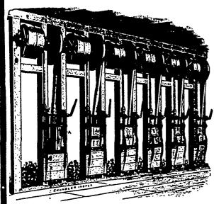
When two or more knives are run with one belt, all must stop when the belt is stopped to set bits or from any other cause. Our Machine has a belt for each knife, hence but one knife stops at a time. This great advantage should not be overlooked by purchasers. Time is money. Our Machine cuts more excelsior in a given time than any other machine. Get our circulars and prices.
