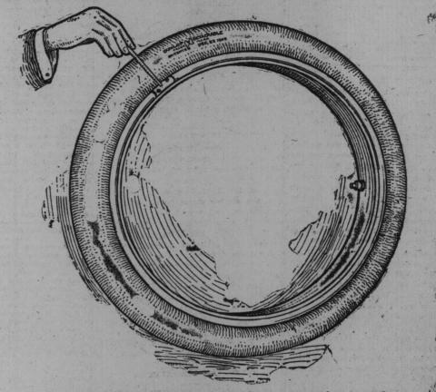
The removable flange is now in place and the operator has inserted a steel pencil in the turn-buckle to tighten it into the groove of channel. This is
