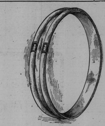
Wheel rim showing turn-buckles in the beads or flanges. The turnbuckles, which join the two ends of the encircling flanges, are fitted with right
