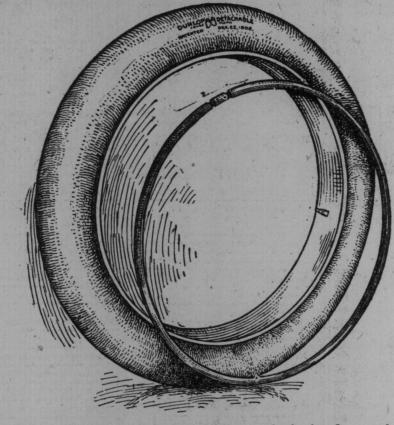
Dunlop Auto Tire on wheel rim showing removable bead or flange ready for attaching. The tire is in place and the flange will slip easily over the edge of
