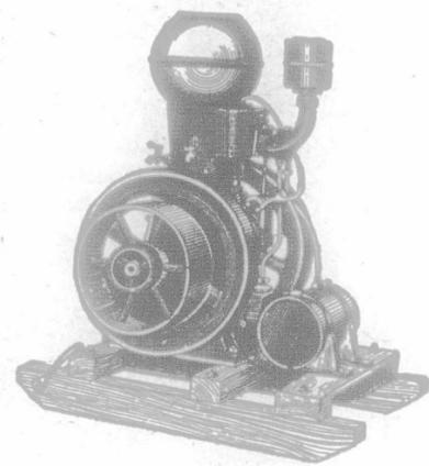
2, 3, 5, 7 and 9 horse power. Standard hopper cooled, throttle governed, automatic lubrication, high tension magneto. "Good old British reliability" throughout.
